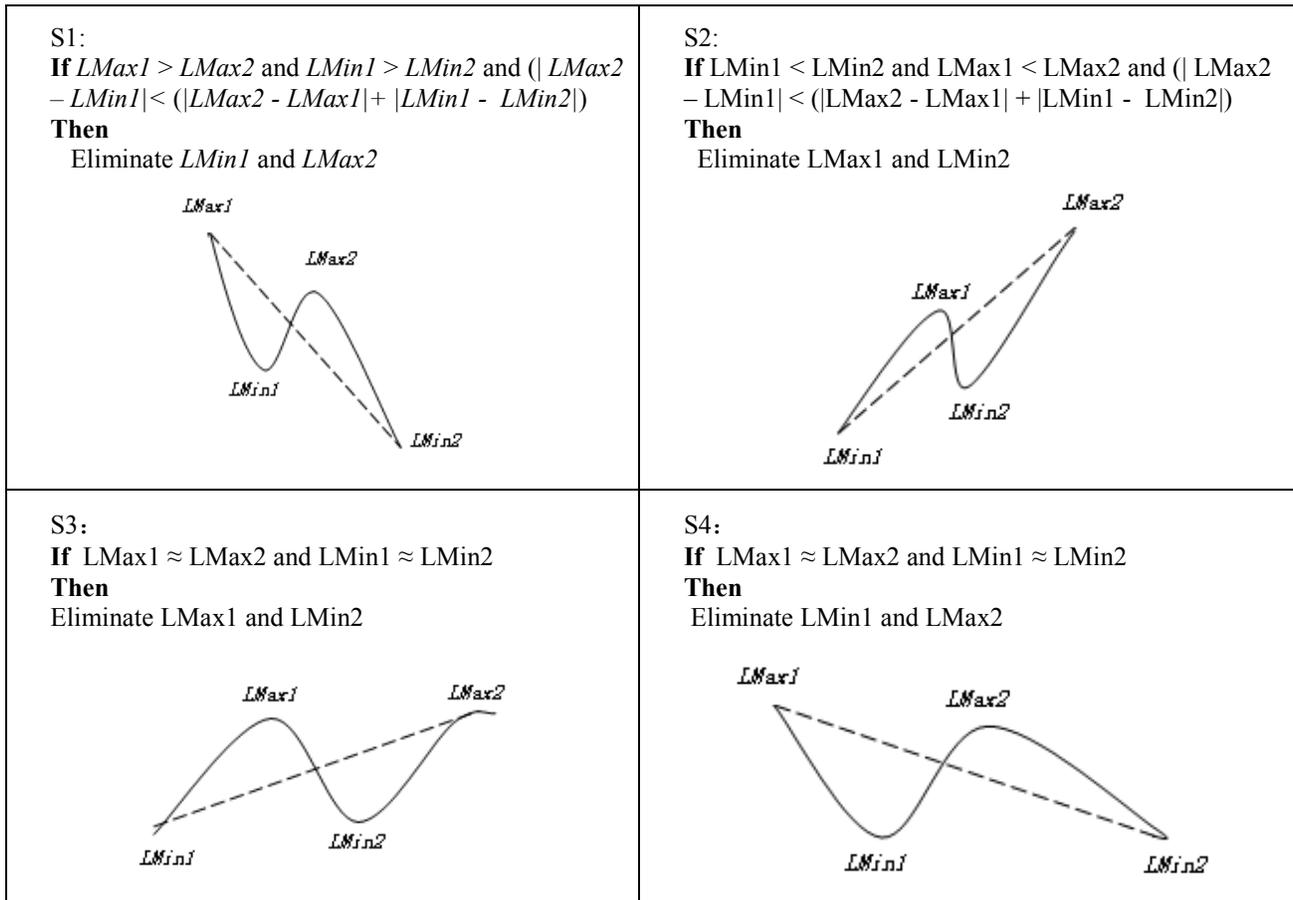
ALGORITHM 2. ALGORITHM FOR GENERATING TURNING POINTS
